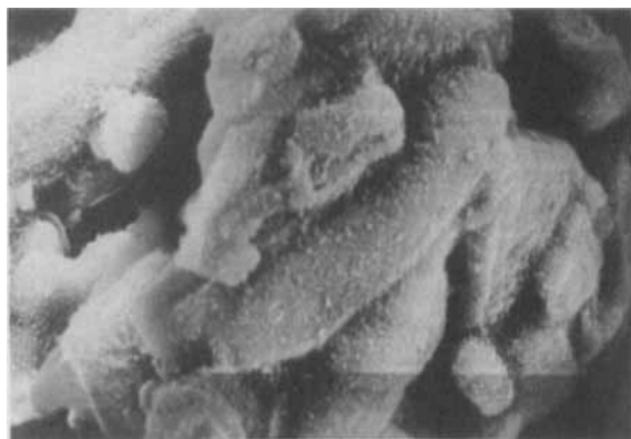
Figure 5. Scanning electron micrograph of dry coated mixture of COMPAP with 0.8% Aerosil® R972.
